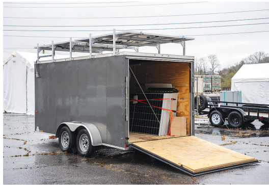
Above: One of Footprint Project's solar microgrid trailers, which offers 20 kilowatt-hours of storage capacity to sustain essential electrical loads during grid outages. Photo by Abby Hassler
