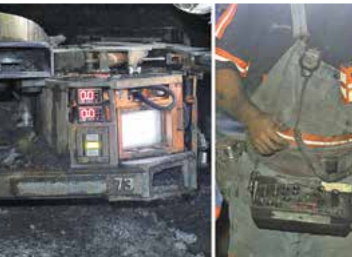
Dust monitors such as these are meant to warn miners of unsafe coal and silica dust levels. Photos courtesy of U.S. Mine Safety and Health Administration
