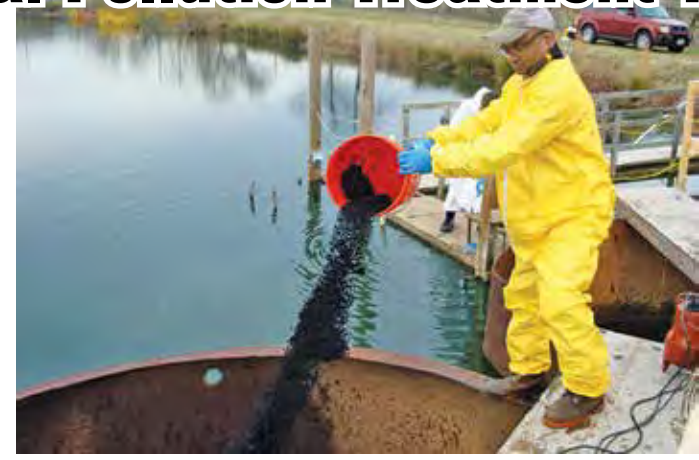
Scientists implement bioremediation techniques in an effort to reduce the volume of PCBs at the overflow pond in Altavista, Va. Photo by Kevin Sowers
