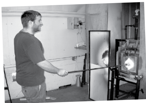
Gas from the Yancey-Mitchell landfill fuels the studios' glass oven. Photos by Energy Xchange
