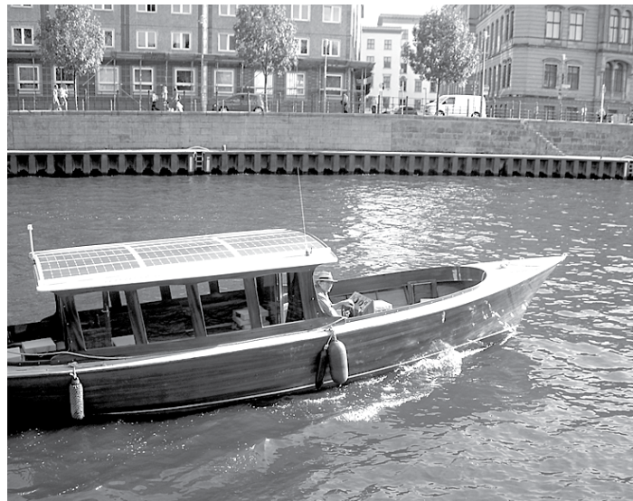
Capt. Arno Paulus pilots a solar photovoltaic boat down the Spree River in Berlin. The boat cruises at about 2-3 knots on one KW of rooftop PV power. Dozens of these boats, and thousands of less photogenic photovoltaic installations, dot Berlin and the German countryside, due in part to strong government subsidies. Photo by Bill Kovarik
