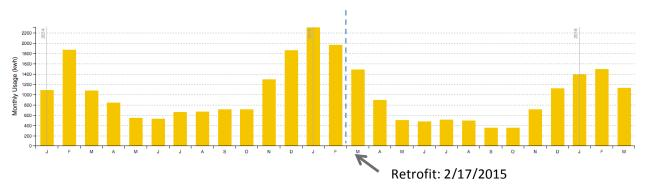
Home #1 shows a baseload electric consumption that reduced from ~550 kWh/month pre-retrofit to ~350 kWh/month post-retrofit. Peak monthly winter usage has dropped from near or above ~2000 kWh/per month to not more than 1500 kWh/month in the post retrofit winter.
