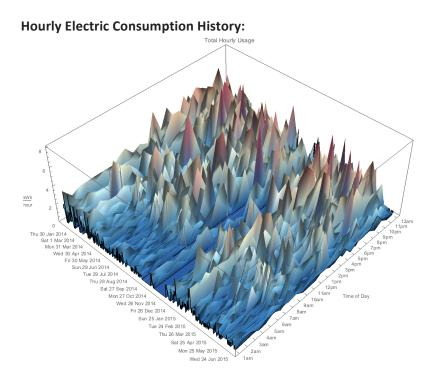
The data reflects electric usage from January 1<sup>st</sup> 2014 though June 27<sup>th</sup> 2015. The home's consumption pattern shows somewhat regular morning ramp-up in the 6-7am meter read, and irregular usage during the day, reflecting the periodic usage of high-watt appliances.
