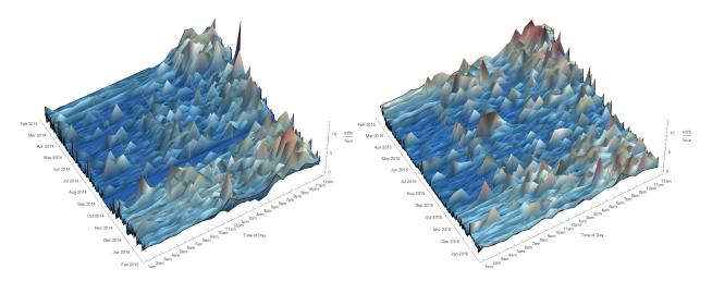
The two plots reflect hourly electric use from 2/18/2014 to 2/17/2015 and 2/18/2015 to 2/17/2016 respectively. Both plots show irregular daily use, with the highest usage in the evening hours, and a high baseline usage (i.e. 24-hour use) from late October through March.
