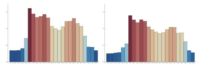
The two plots reflect hourly electric use averages from 3/2/2014 to 3/1/2015 and 3/3/2015 to 3/1/2016 respectively. Both plots show regular daily usage between 6am and 9pm, with peak use reduced from an average of 1.6 to 1.4 kWh/hour, morning use in the subsequent hours reduced from ~1.4 to ~1.25 kWh/hour, and overnight use reduced from ~0.35 to ~0.27 kWh/hour.
