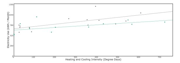
The home shows a reduction in heating performance index from 0.43 kWh/ $^{0}$ F-day pre-retrofit to 0.34 kWh/ $^{0}$ F-day post-retrofit. The weather-corrected pre-retrofit model indicates ~850 kWh of electricity not used in the 13 post-retrofit months analyzed, an 8% savings.
