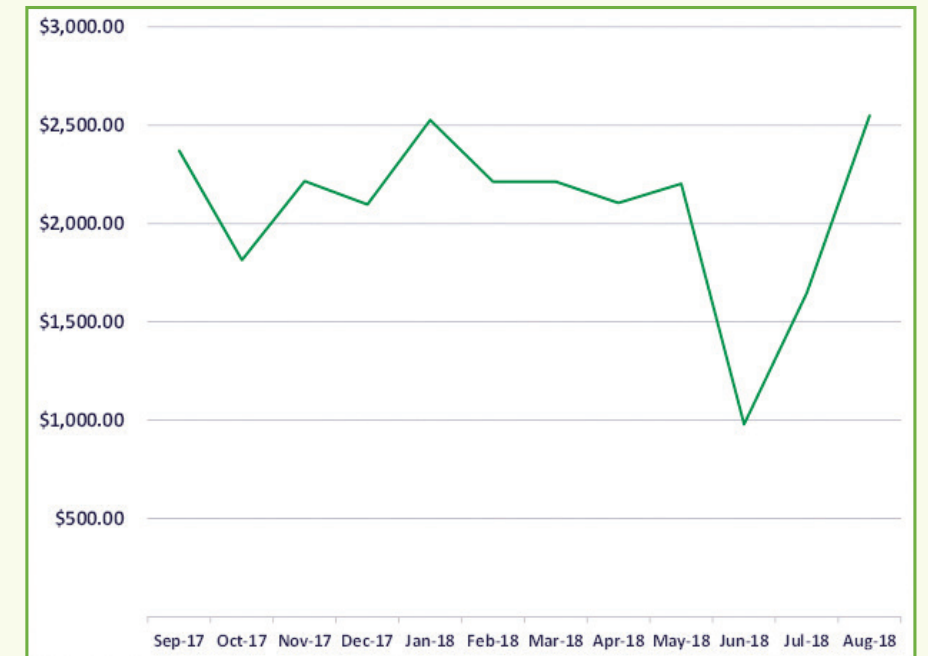
Figure 2: Electricity consumption at Arlie Boggs Elementary, September 2017 to August 2018.
